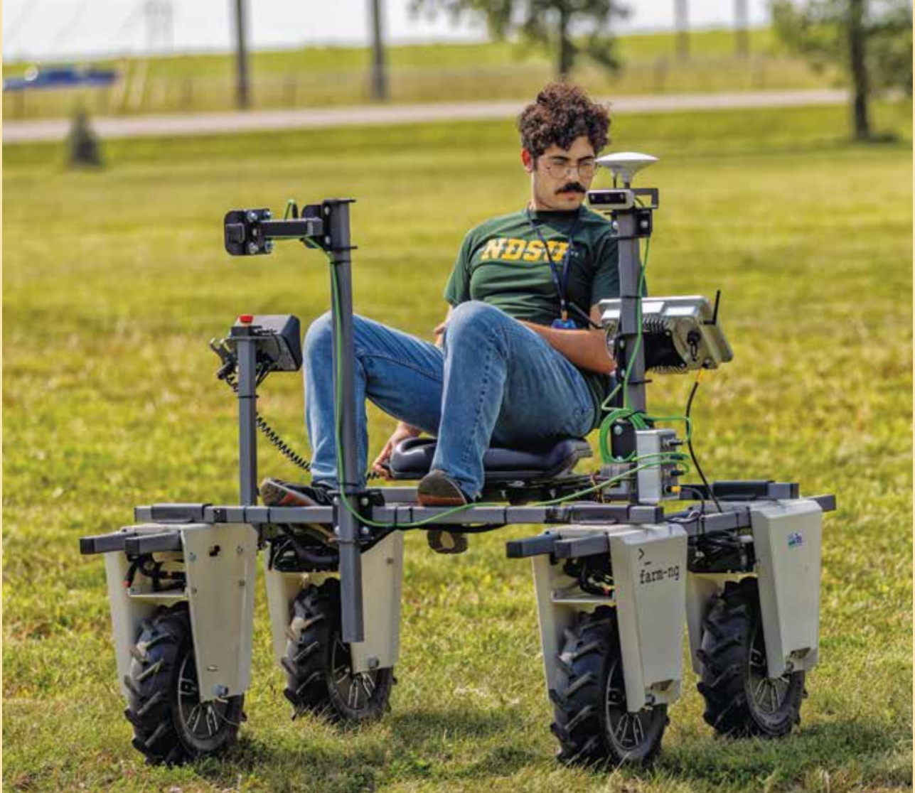
An NDSU graduate student demonstrating the Amiga Robot, an all-electric micro-tractor. This work is led by James Kim, PhD, a research scientist at USDA Agricultural Research Service in Fargo and an Adjunct Professor at NDSU's Agricultural & Biosystems Engineering. Prof. Kim uses the robot for research on engineering solutions for crop protection with UAS-based field mapping for AI-based target identification and a robotic platform for field scouting and treatment.
